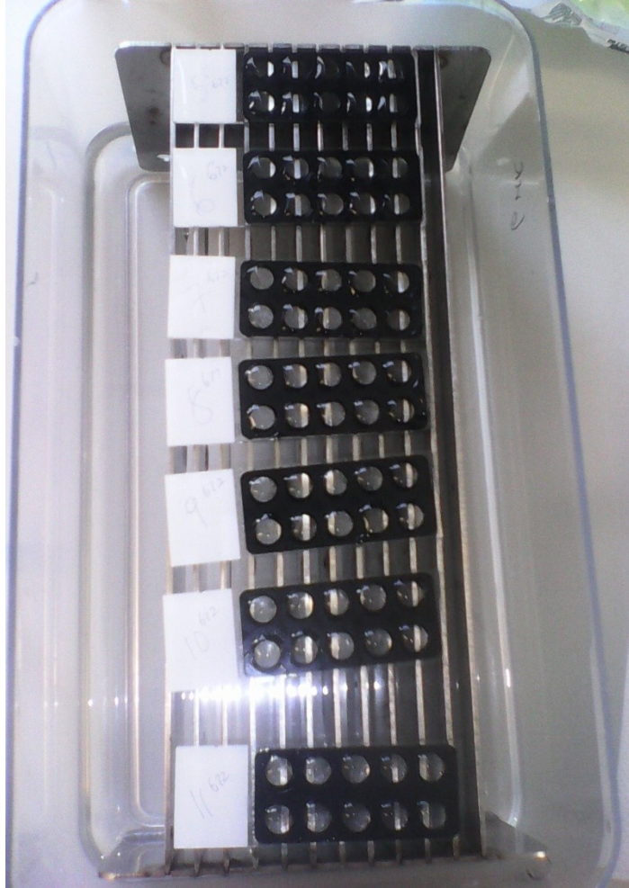
Plate 3.1: Multispot slides with test samples placed on staining rack in humidified chamber
