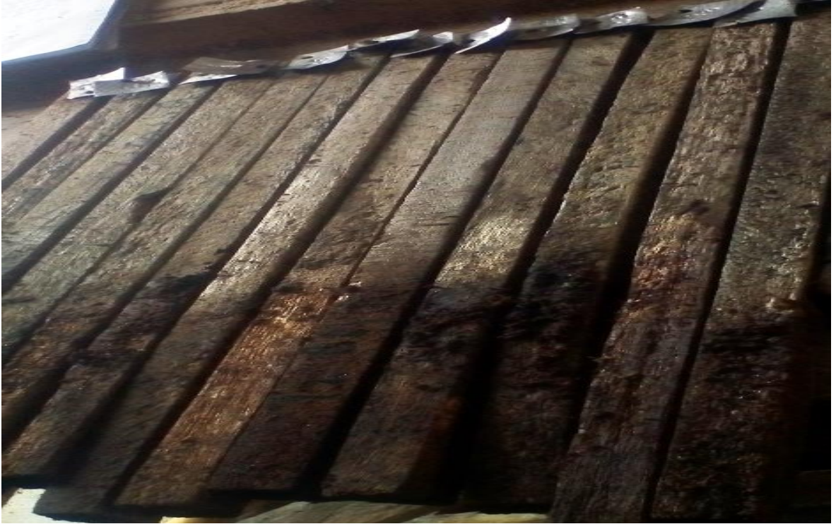
Plate 4.7: Visual observation of moderately attacked wood samples of A. altilis
