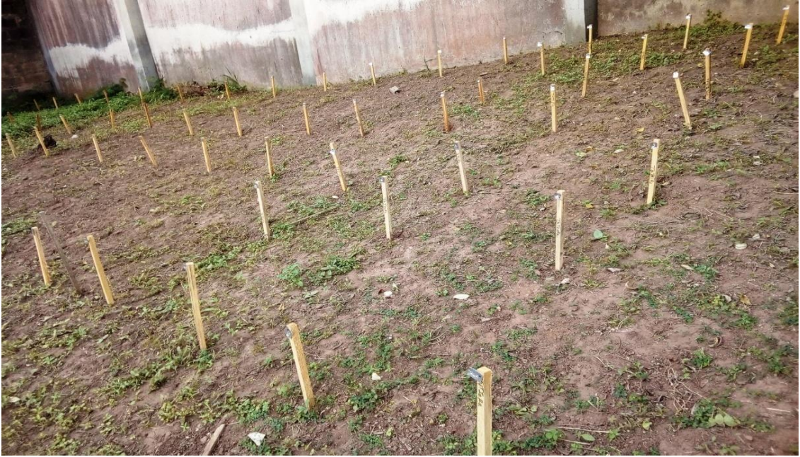
Plate 4.6: Test samples buried at the Timber Graveyard at 25% of sample height and at 1m x 1m interval on the field.
