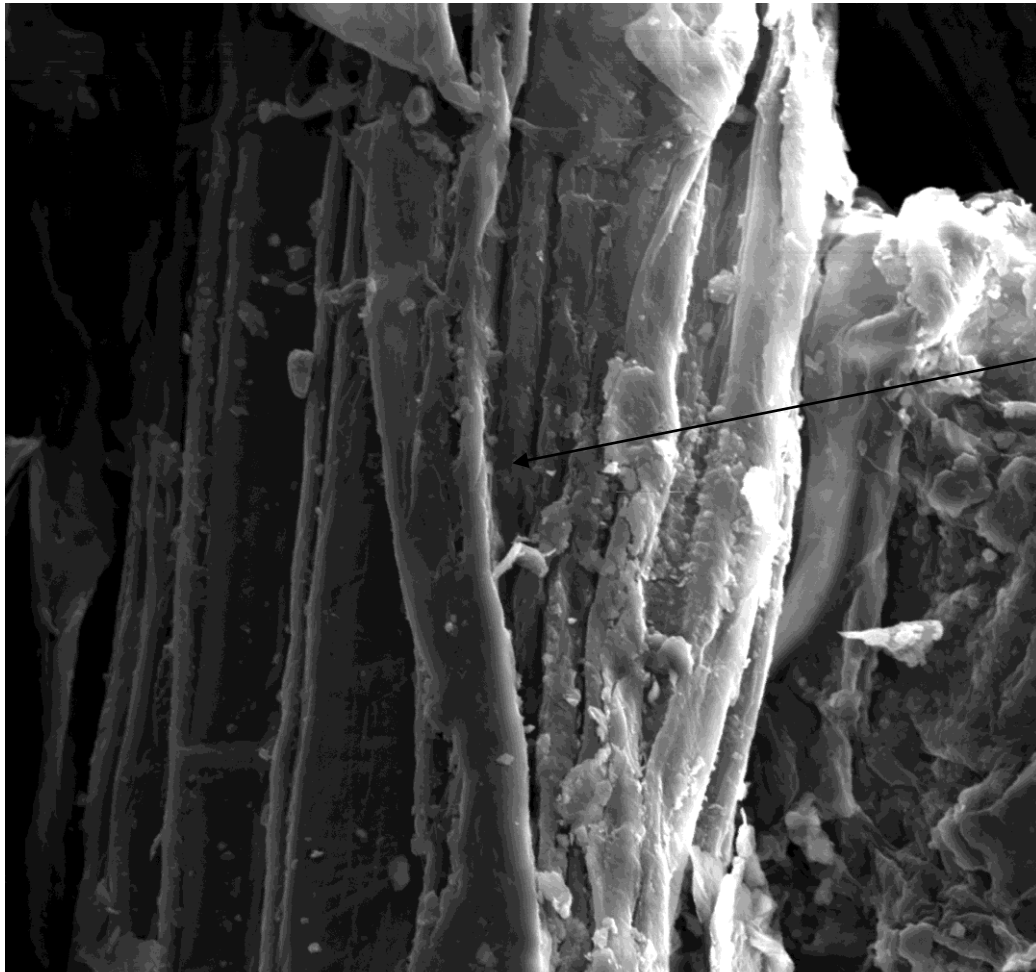
Plate 4.2: Scanning electron micrograph of pretreated bagasse showing mainly the fiber structure
