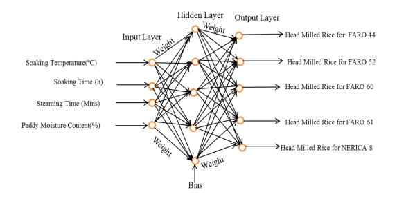
Fig. 4.16. The optimum architecture of the developed ANN model for head milled rice
