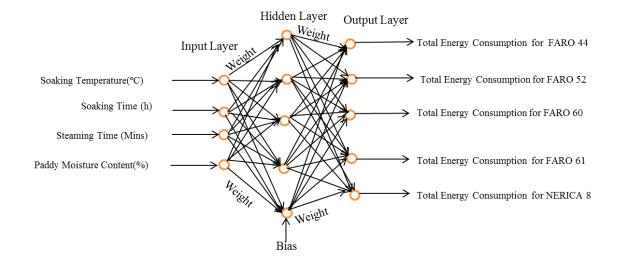
Fig. 4.4. The optimum architecture of the developed ANN model for total energy consumption
