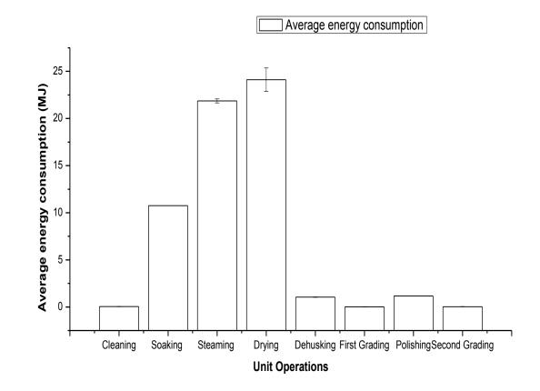
Fig. 4.3. Average energy consumption pattern in processing paddy rice into polished parboiled rice
