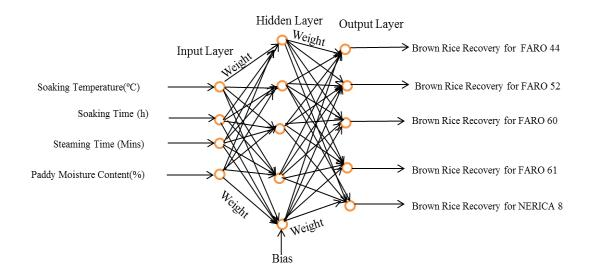
Fig. 4.7. The optimum architecture of the developed ANN model for brown rice recovery
