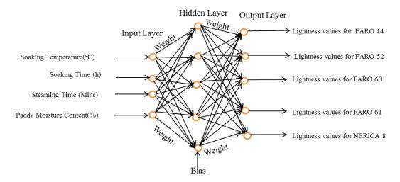
Fig. 4.22. The optimum architecture of the developed ANN model for lightness
