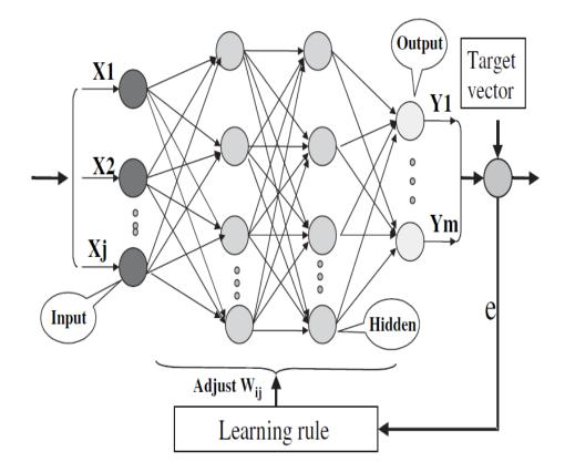
Fig. 2.3. Atypical multi-layer Artificial Neural Network (Chen et al. 2007)
