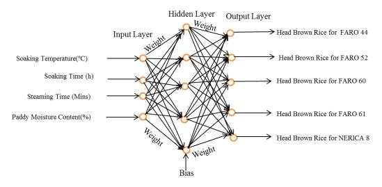
Fig. 4.10. The optimum architecture of the developed ANN model for brown rice recovery
