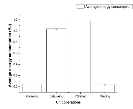
Fig. 4.1. Average energy intensity pattern in processing paddy rice into white rice
