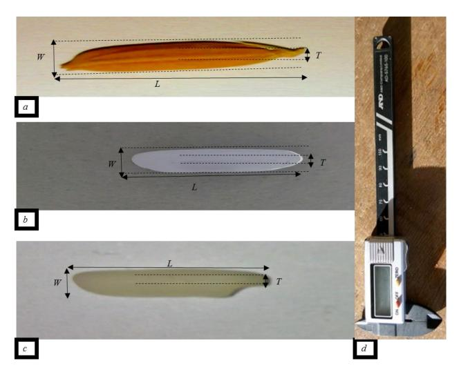
Plate 3.1. Paddy grain (a), White rice (b) and Parboiled polished rice (c) axial dimensions and digital vernier caliper (d)
