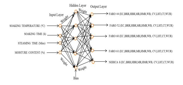
Fig. 3.3. Schematic diagram of the developed feedforward multi-layer ANN
