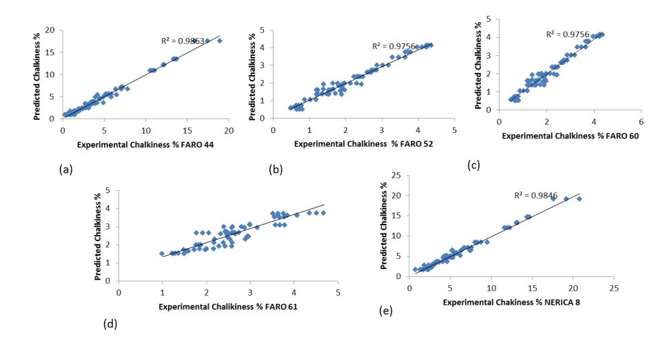
Fig. 4.21. Comparison between the experimental chalkiness and predicted chalkiness using ANN
