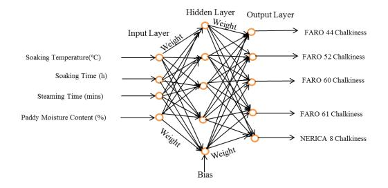
Fig. 4.19. The optimum architecture of the developed ANN model for chalkiness
