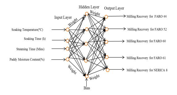
Fig. 4.13. The optimum architecture of the developed ANN model for milling recovery
