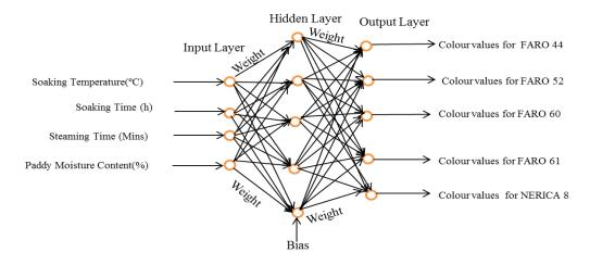
Fig. 4.25. The optimum architecture of the developed ANN model for colour
