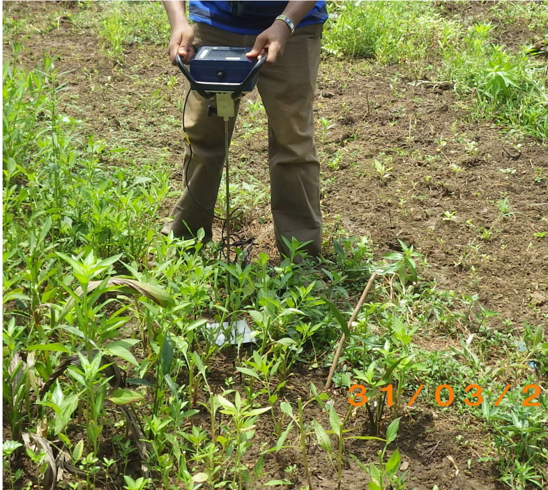
Plate 3.1 Penetration resistance reading taken at an urban agriculture site at Okitipupa
