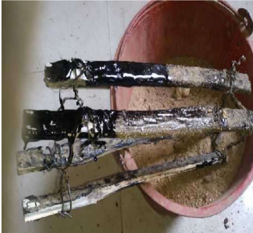
Plate 3. 40: Coating treated bamboo reinforcement with fine sand
