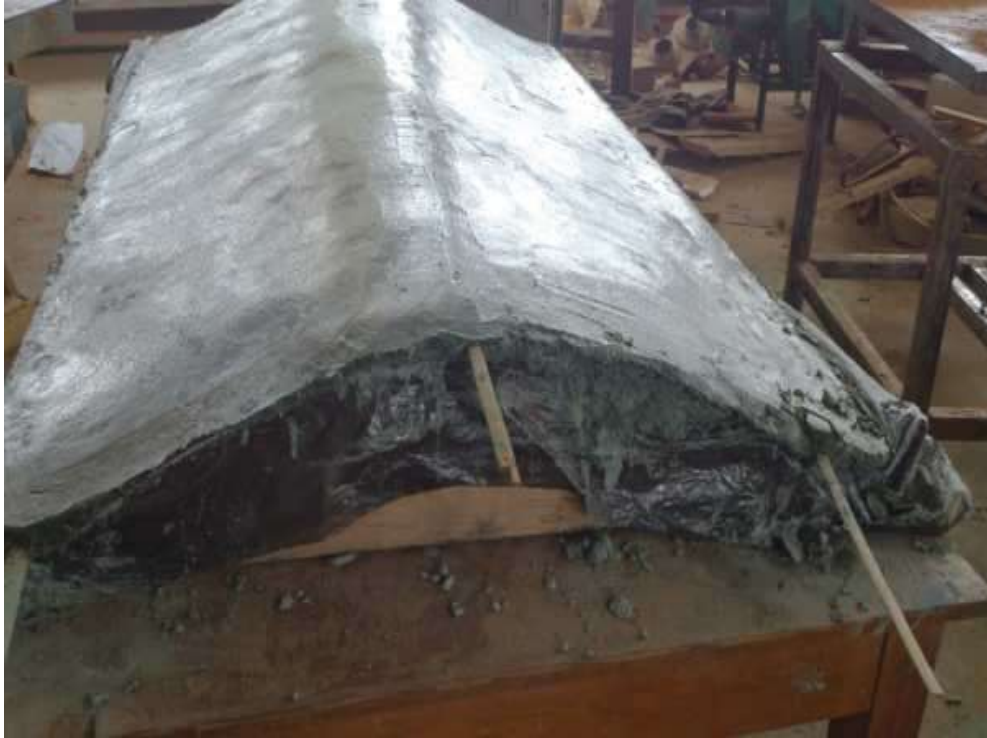
Plate 3.8: Developed composite roofplaced onwork table
