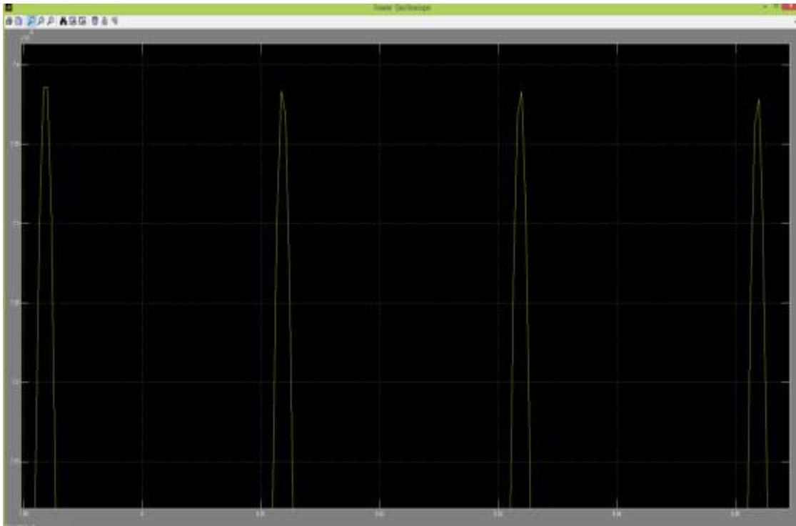
Figure 4.14: Result showing the Output Bus Voltage at Fowler to be 73.80V with the implementation of two RLC Band pass Filters in Cascade
