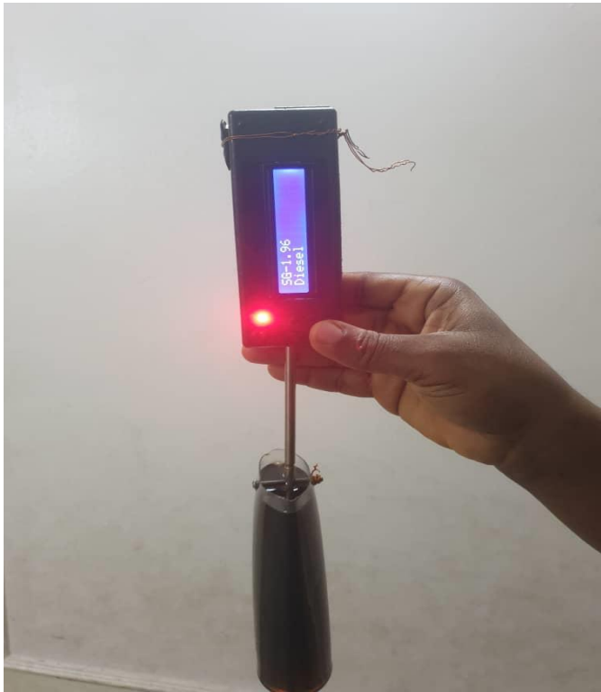
Figure 3.20: Adulterate - meter detecting Impurity in Diesel
