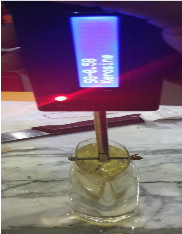
Figure 3.21: Adulterate - meter detecting Impurity in Kerosene.
