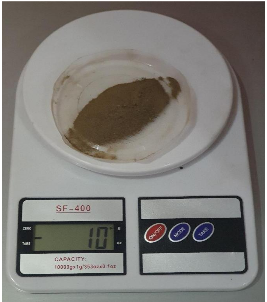
Figure 3.5: Scale Measuring Sand dust in a Petri dish
