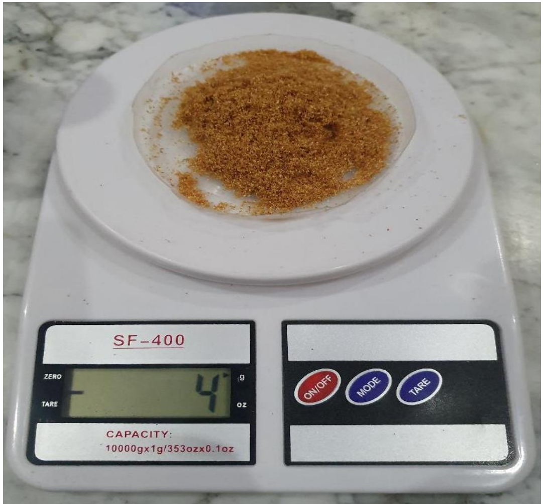
Figure 3.6: Scale Measuring Sawdust in a Petri dish
