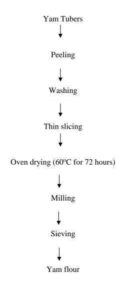
Figure 3.1. Flowchart for yam flour preparation Source: Wireko-Manu *et al.*, 2011
