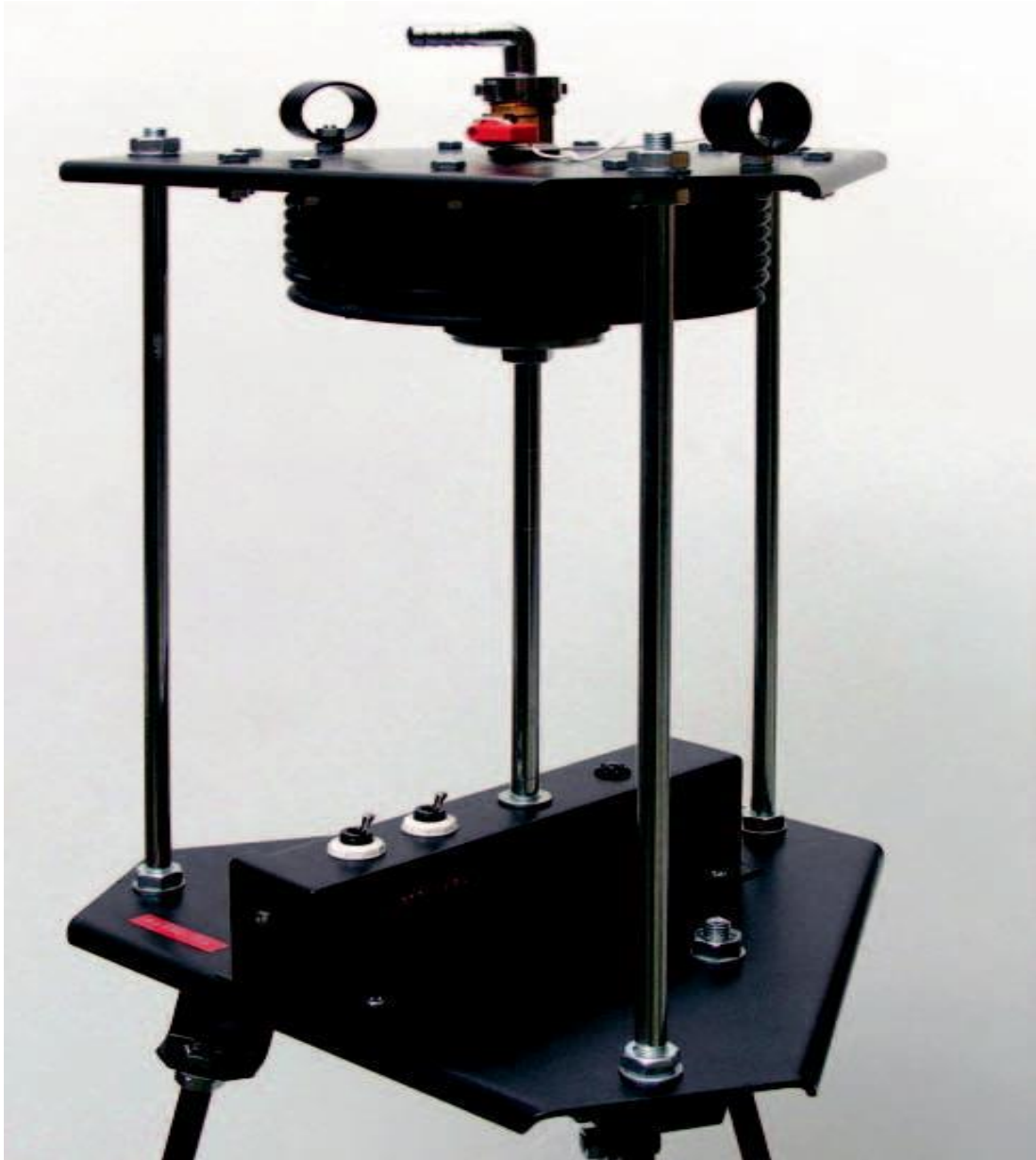
Plate 2.2 RADON-JOK Equipment for in situ Soil-air Permeability Measurement (Mezon, 2017)
