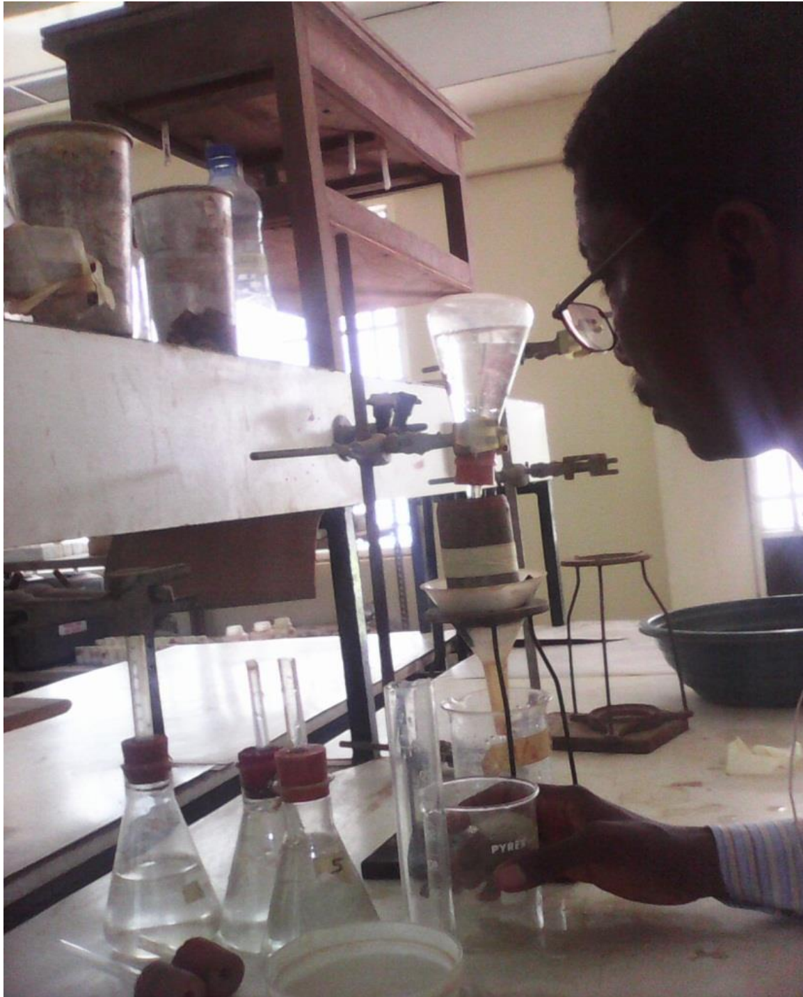
Plate 3.1 Constant head permeameter set-up for measurement of saturated hydraulic conductivity
