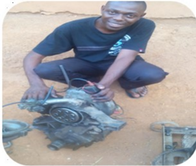
Plate 3.10: Starter coil removed for CVT to be attached to the crankshaft
