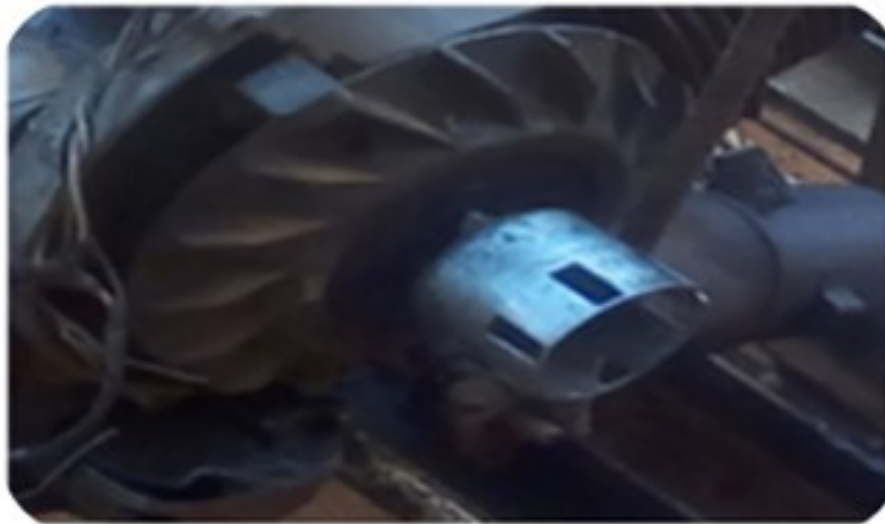
Plate 3.11: The starter hub improvised for engine cranking
