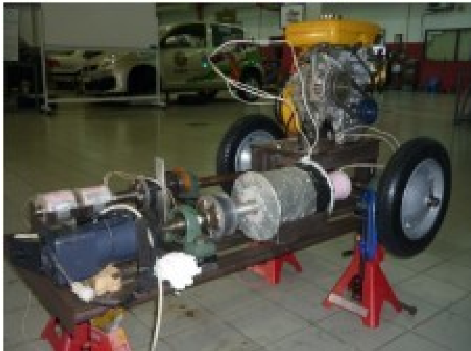
Fig 2.13: An Electromechanically Actuated CVT System (Rahman et al. , 2014)
