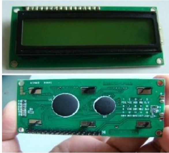
16-pin LCD, Pin 15 Led+ and Pin 16 is LED-
