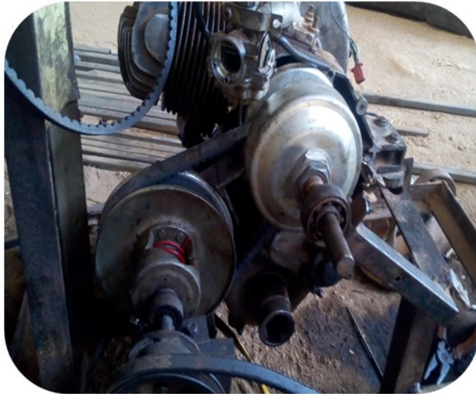
Plate 3.12: CVT retrofitted autorickshaw engine
