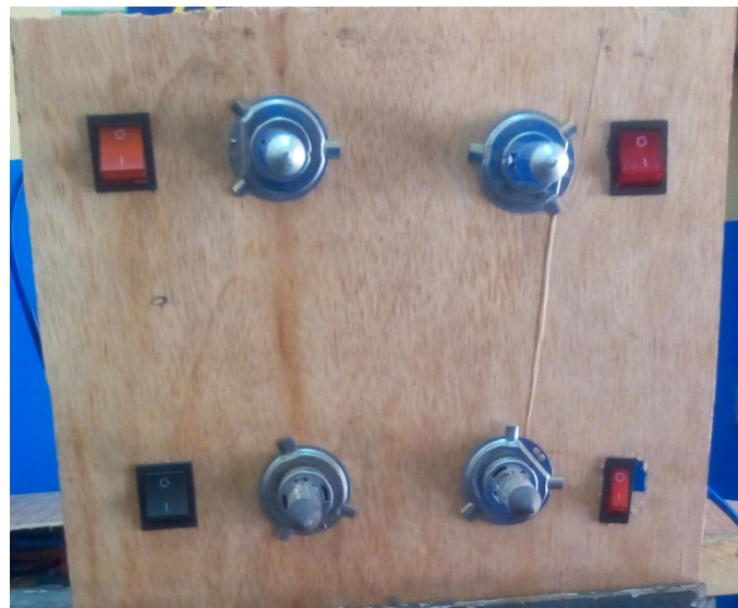
Plate 3.14b: Load Variator 2 (800W loads)
