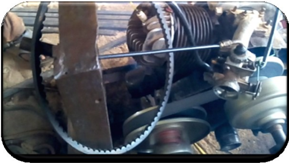
Plate 3.20: CVT at lowest ratio
