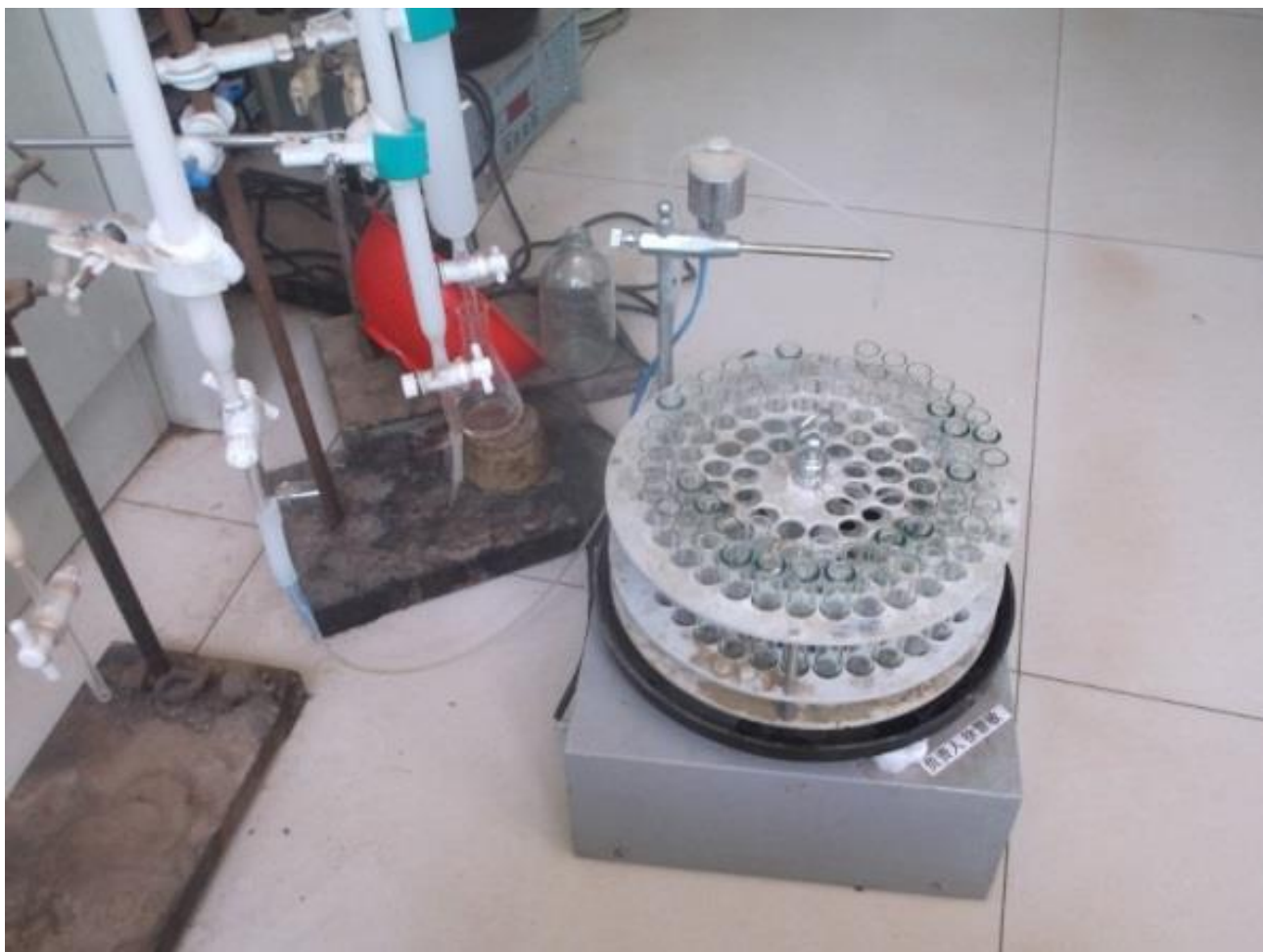
Figure 5.5: A picture showing the collection of sub-fractions of ethanol extract of Grewia carpinifolia using an open column chromatography with an automated fraction collector
