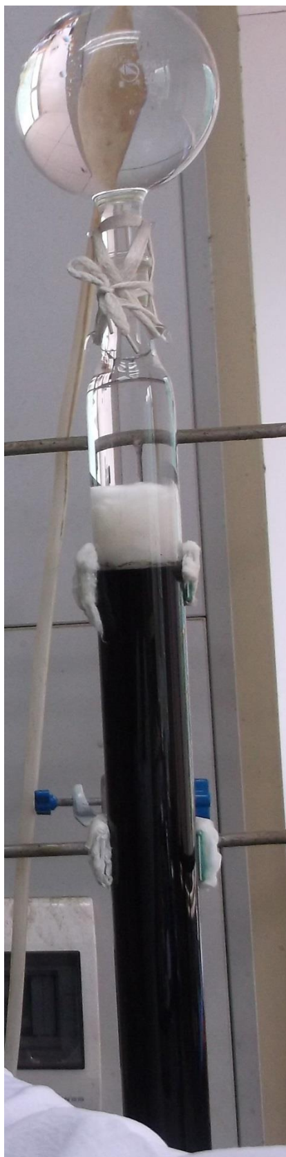
Figure 5.4: Purification of the ethanol extract of Grewia carpinifolia using the column chromatography
