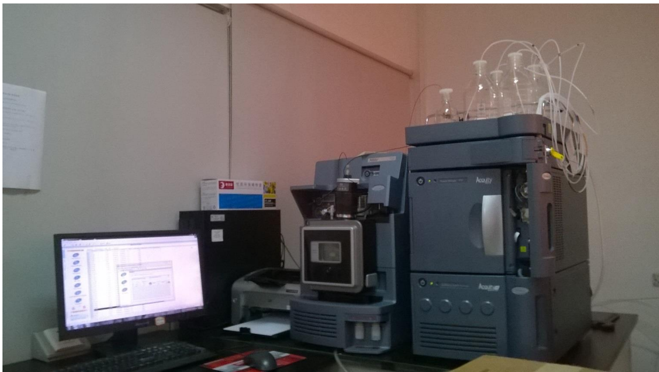
Figure 5.6.: A picture of the High Performance Liquid Chromatography (HPLC) equipment
