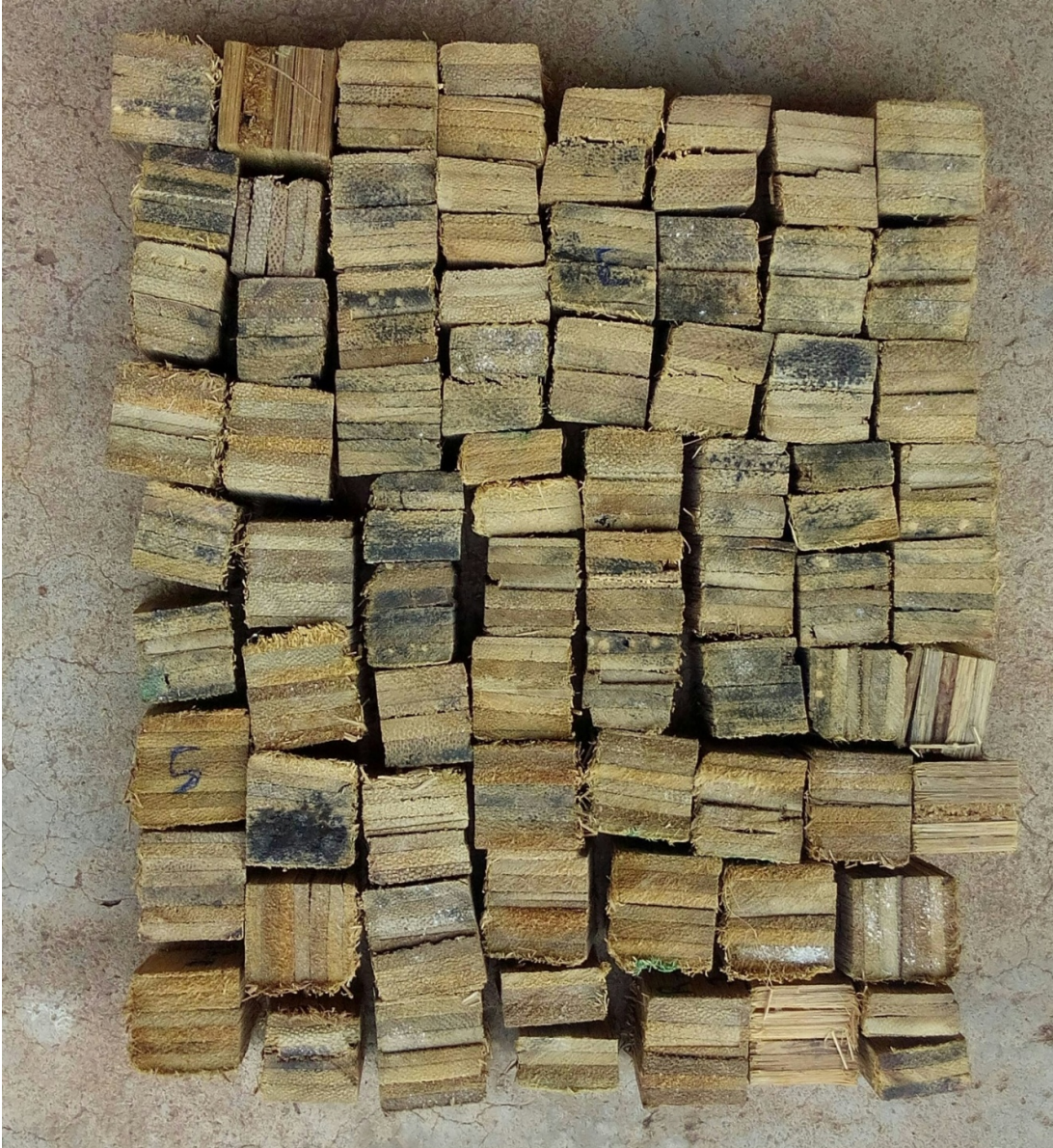
Plate 3.6 Failed Shears samples of Glulam Bambusa vulgaris along the glue lines
