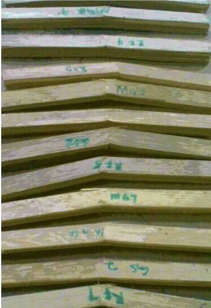
Plate 3.4 Failure Patterns of Some MOR and MOE Test Samples of Glulam Bambusa vulgaris
