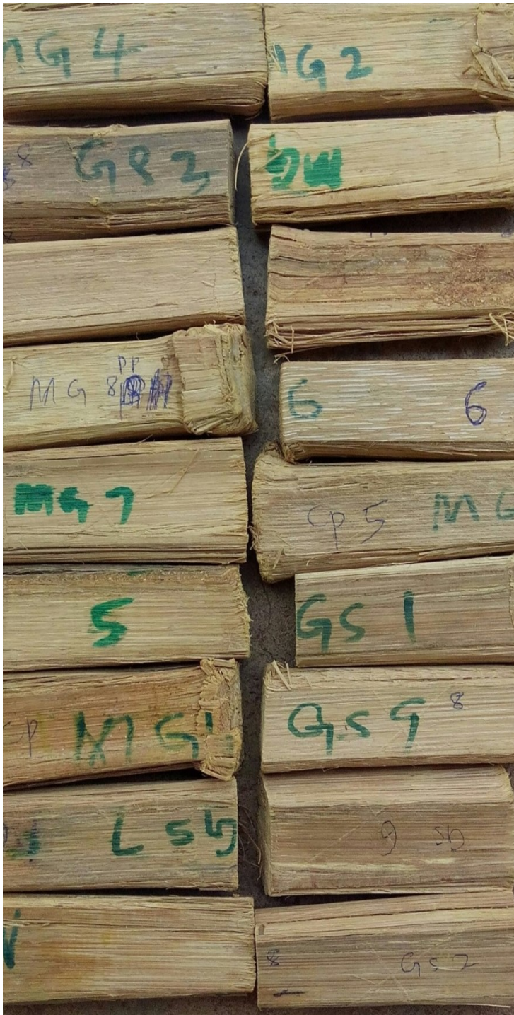
Plate 3.5 Failure patterns of Some Samples of MCS Parallel and Perpendicular to Grain of Glulam Bambusa vulgaris Glulam.
